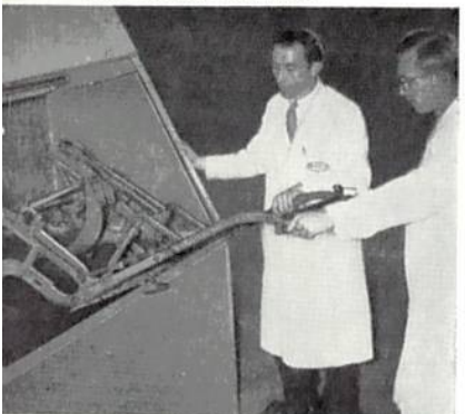
All the old painted parts are cleaned down to the bare metal in a chemical bath in preparation for repainting. Extractor fans are used to exhaust fumes out of the factory.
