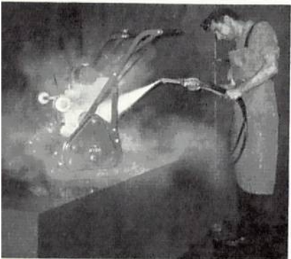
A high pressure paraffin jet cleans off all the caked oil, grease and dirt prior to the machine being dismantled for overhaul.
