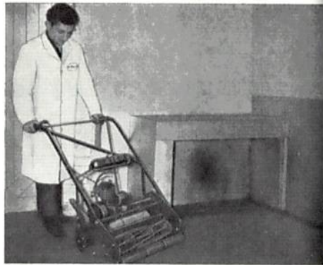
The final running tests are carried out in an air conditioned cubicle where an extractor fan carries the harmful exhaust fumes beyond the factory walls. From here the passed out machine is loaded on to Atco transport for redelivery to the User.
